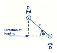
Note 3: For all of the above reduction factors, if different size piers are used in a group, D used in the above formulas should be the largest pier diameter in the group.
