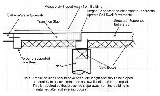
All void spaces should be drained. We recommend that Alliance Geotechnical Group be retained to review the project drawings and specifications to ensure compliance with the geotechnical report.
