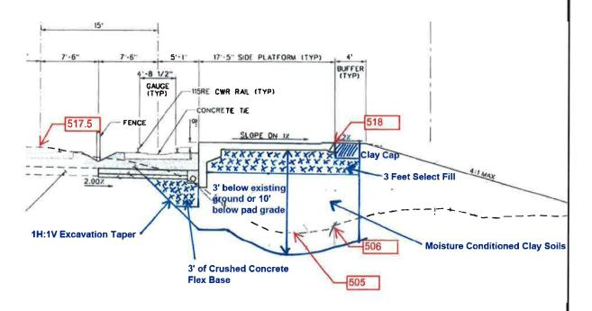
The excavation limits should extend at least 20 feet beyond building lines and then transitioned on 2H:1V slope at track entrances into the platform. These excavation extensions will be limited as described above and as shown in the above schematic.
